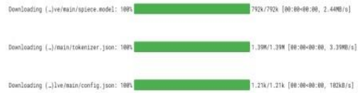
Fig 3. The code is downloading model files from some source. These files include the vocabulary (spiece.model), tokenizer information (tokenizer.json), and model configuration (config.json) for the T5 model.
